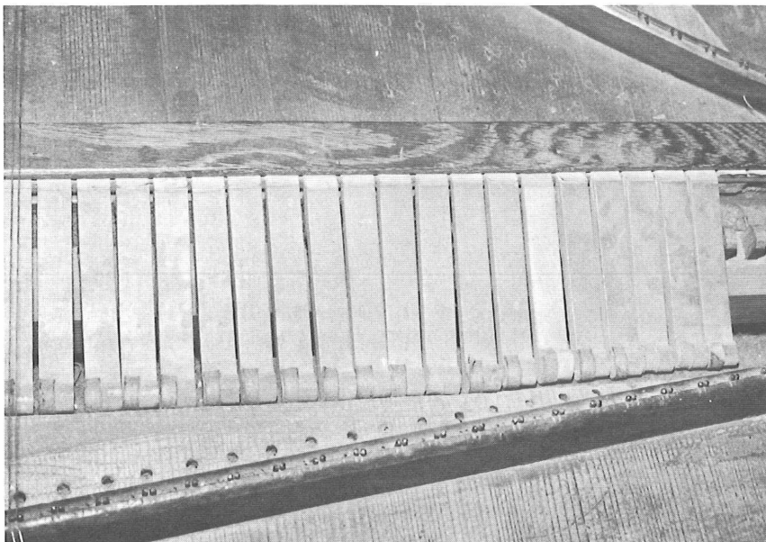
Illustration 2. Anonymous German harpsichord with later hammer action (Musical Instrument Museum of the National Museum, Poznan): detail of hammers with leathered and bare wood striking surfaces.
