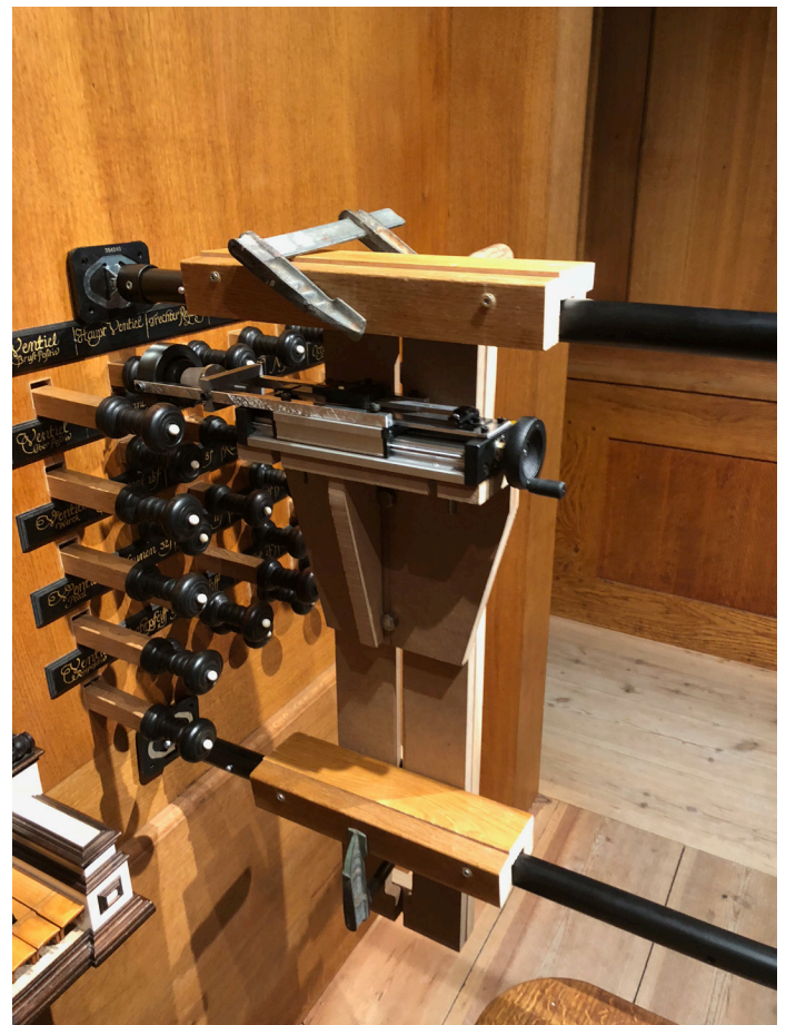
Detail showing the device we built to allow Ericsson to close the Hauptventil one millimeter at a time.
